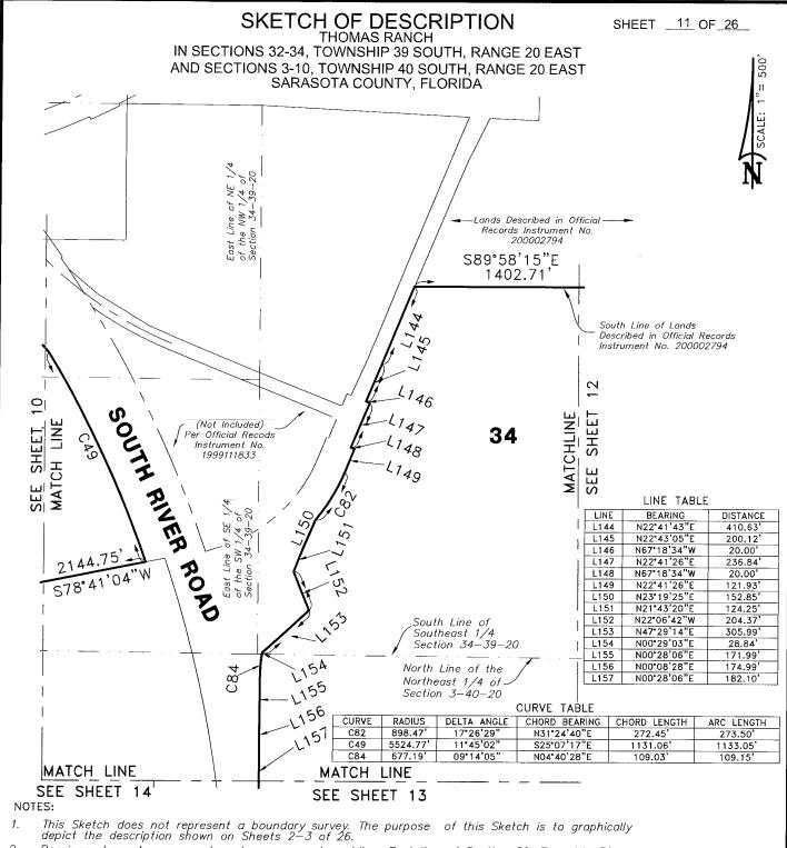
Bearings shown hereon are based an assumed meridian. East line of Section 29, Township 39 South, Range 20 East = N.02\*49'06"W.
